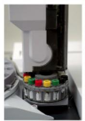
Autosamplers extracting the sample from the vial with a syringe, need the syringe rinsed after each injection to keep sample carryover at a minimum. With increasing sensitivity of the Analysis, the rinsing process becomes increasingly important, especially when different or viscous samples are analysed. The vial in which the solvent is kept is the so called Wash Vial.
