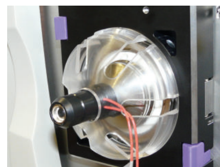
Figure 2 - SICRIT® setup (SC-20 ionization set) with MS interface, ion source and control unit (top). SICRIT® ion source, interlock and safety cap (TX2 interface) attached to a Thermo MS API inlet (bottom).
