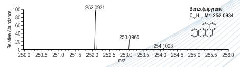
Diagram 1: Accurate mass spectra of Benzo(a)pyrene
