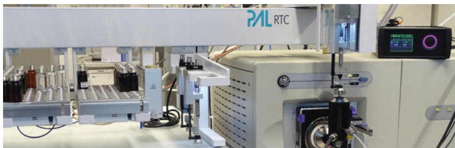
Figure 2 - Automated direct SPME-MS analysis using a PAL RTC sample preparation system and a SICRIT ® SPME desorption module installed at a Thermo API MS inlet.
