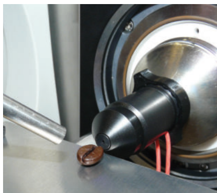
Figure 2 -Coffee aroma profiling by direct VOC desorption in front of the SICRIT® ion source
